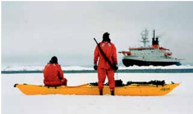
**Fig. 11:** Ice thickness measurements during ARK XVII/1, using a ground-based EM instrument housed in a kayak (Photo: J. Bareiss).
